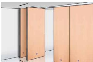
Move the panel (No. 2) until the top roller reaches the branch track whilst pushing the top roller into the branch track. You can then move the panel into its final parking position.
