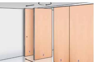
Turn the panel through 90 degrees. You can then move it into its final parking position.
