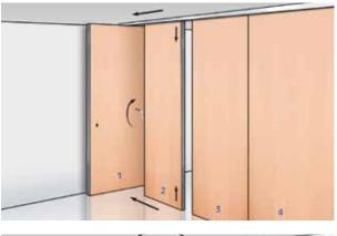
Push the panel (No. 1) at right angles to the track into its final parking position. To unlock the next panel (No. 2), insert the crank handle into the socket in the rear profile of the panel and turn it anti-clockwise until it stops. The horizontal seals retract and you can pull the panel out from its joint with panel 3.
