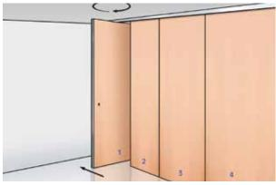
You can now pull panel 1 out from its joint with panel 2. Use the crank handle to help with this movement. Now turn the panel through 90 degrees.
