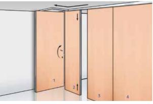
Move the telescopic panel (No. 1) into its final parking position. To unlock the next panel (No. 2), insert the crank handle into the socket in the rear profile of the panel and turn it anti-clockwise until it stops. The horizontal seals retract and you can pull the panel out from its joint with panel 3.
