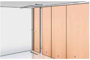
You can now pull panel 1 out from its joint with panel 2. Use the crank handle to help with this movement. Move panel 1 until the top roller reaches the branch track whilst pushing the top roller into the branch track
