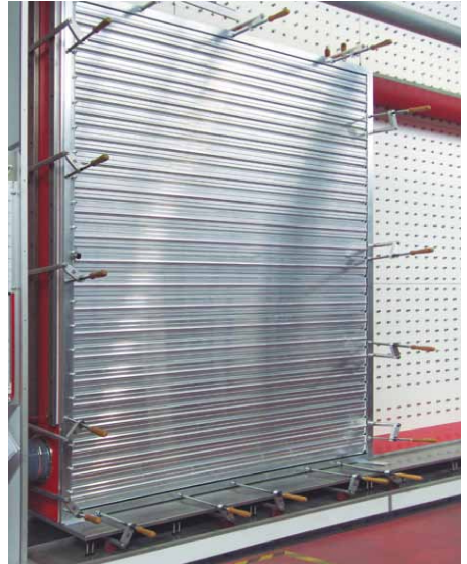
Testing the wind resistance of the AC-150 slat in the Giménez Ganga laboratory.
